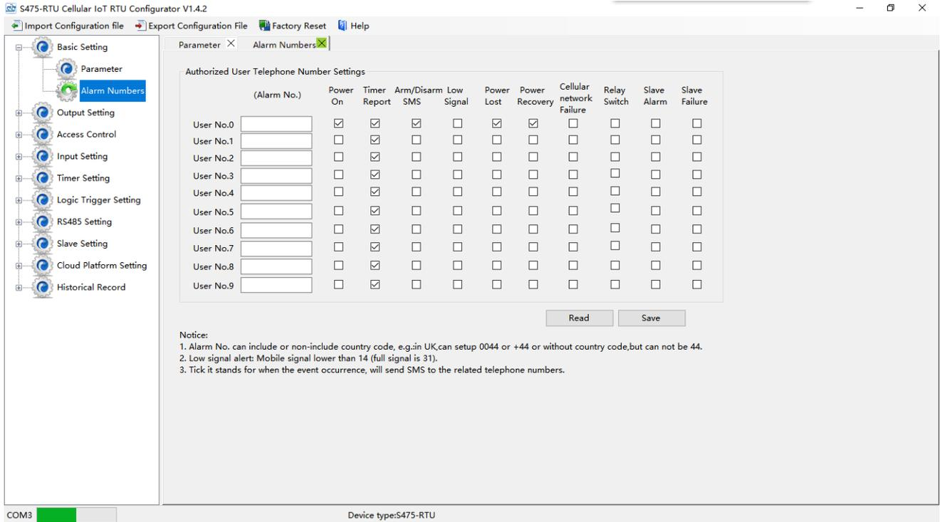
Then switch off the device, insert sim card, switch on the device. after the device register network successfully, the phone number can receive SMS sent by the device. If you cut off the device power, the phone number will receive power failure SMS sent by the device.... That shows the device work normally.
