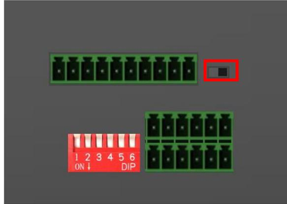
**Power Switch** For switch ON/OFF the RTU
