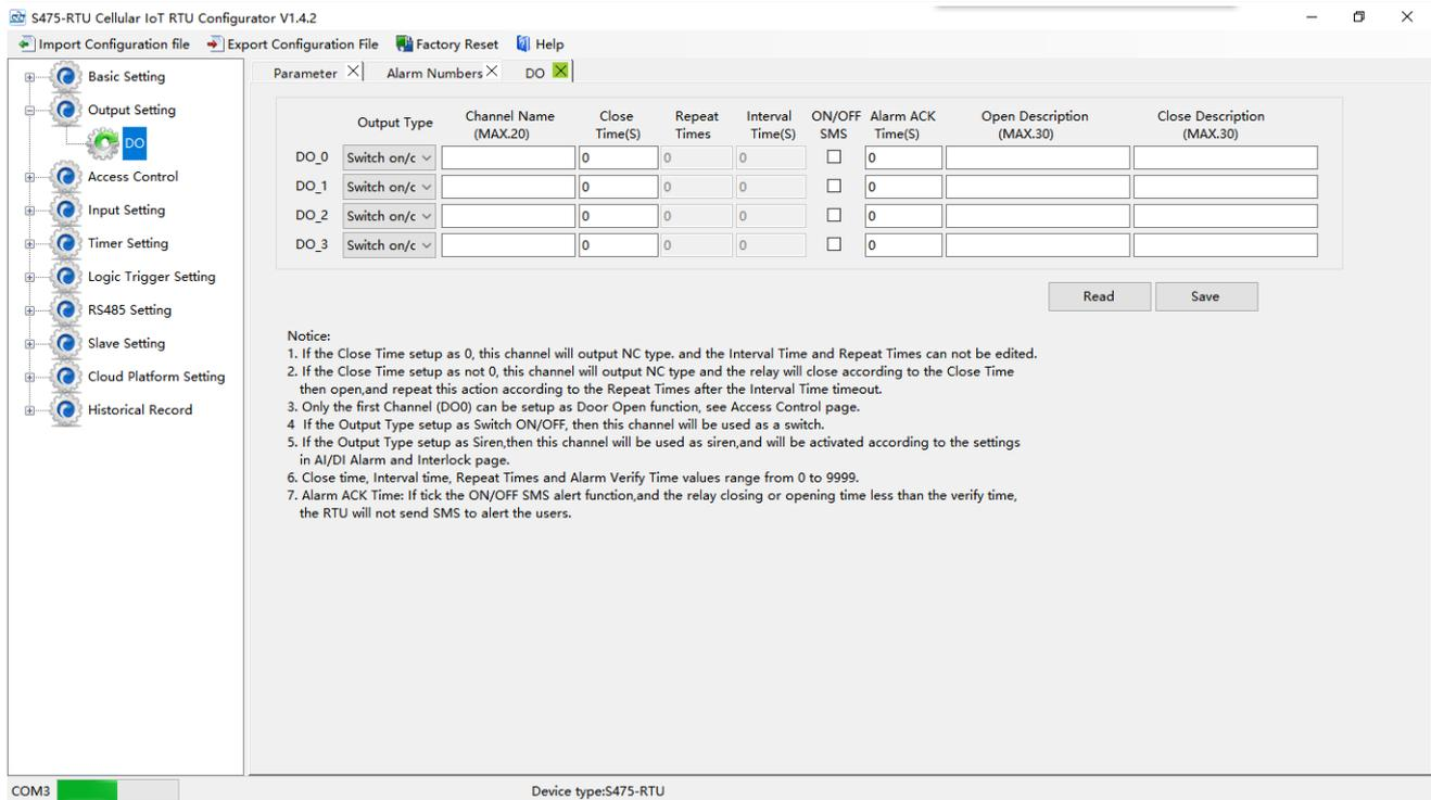
**Output Type:** Support 3 output types. The user can choose the output type for the relay outputs, includes Open Door, Switch ON/OFF, Siren. The relay 2 and 3 only used for Switch ON/OFF; Relay 0 can option as Open Door and Switch ON/OFF; Relay 1 can option as Siren and Switch ON/OFF.
