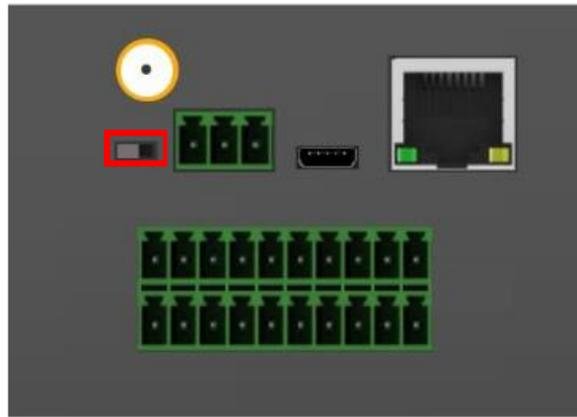
**Upgrade Firmware Switch** For upgrade firmware purpose only. Only when upgrade new firmware version will use it, otherwise keep it at Work Side all the time.
