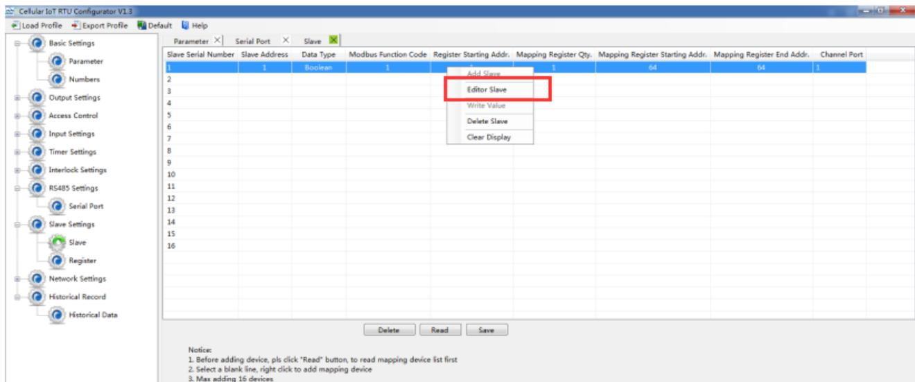
Click the "Editor Slave" to set channel name, alarm SMS content, recovery SMS content and relay active etc. as below:
