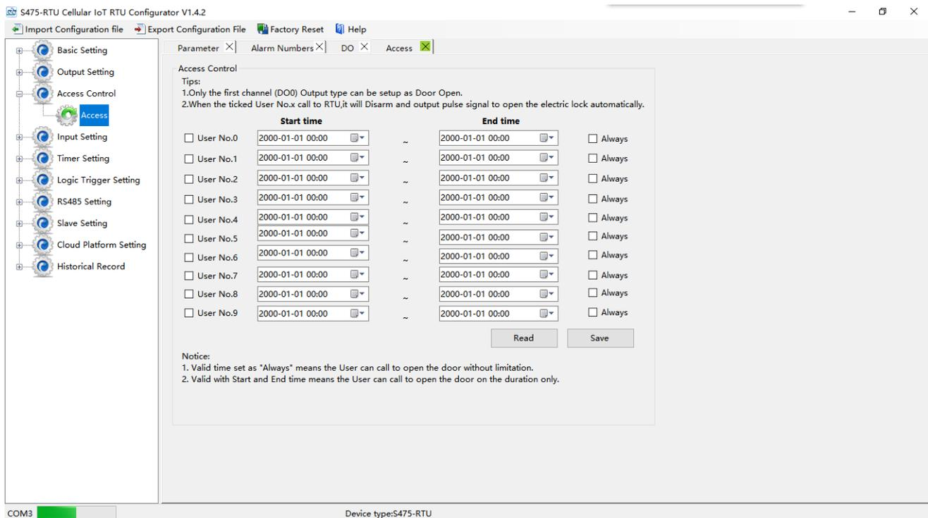
The screenshot shows the 'Access Control' configuration window. It includes a sidebar with navigation options like Basic Setting, Output Setting, Access Control, and Access. The main area is titled 'Access Control' and contains a table for configuring user access. Below the table are 'Read' and 'Save' buttons and a 'Notice' section.
