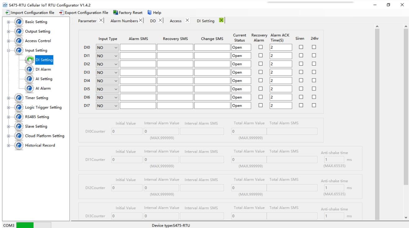
**Input Type:** The user can choose the input type for related channel. Includes: Counter, Arm/Disarm, NC, NO, Change and Disabled.
