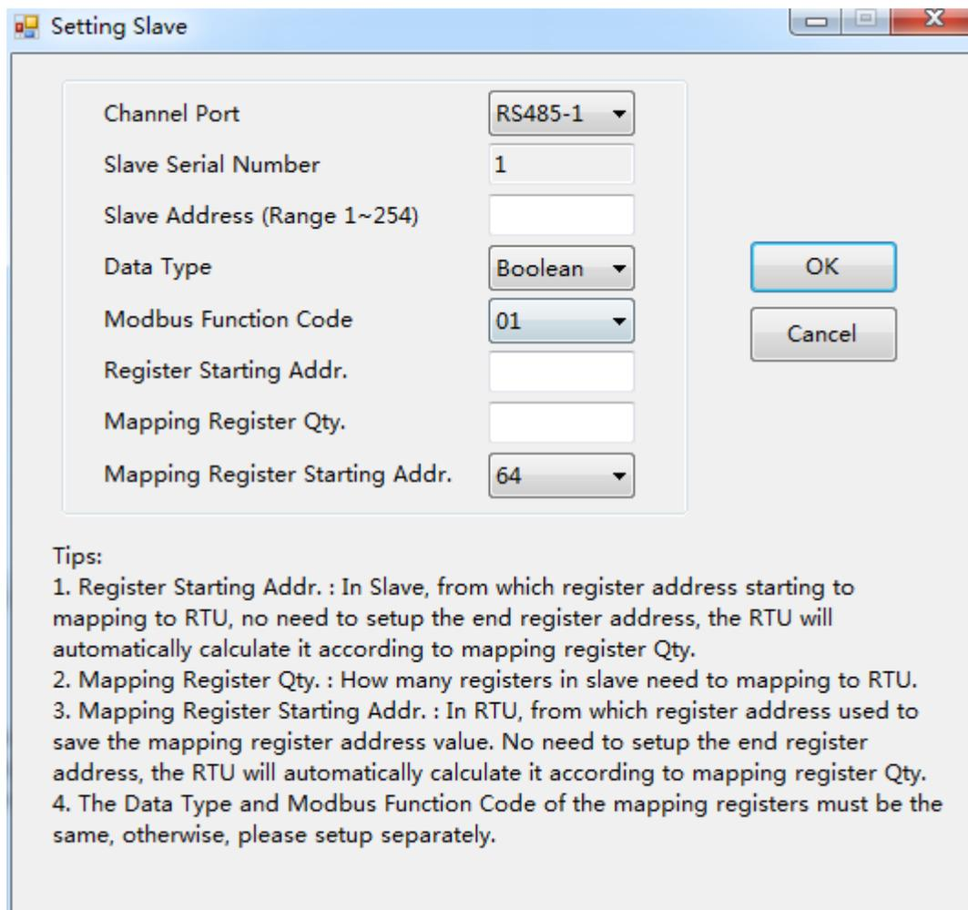
If one slave have multi register, then need to add separately according to register type; For example, Mxxx
