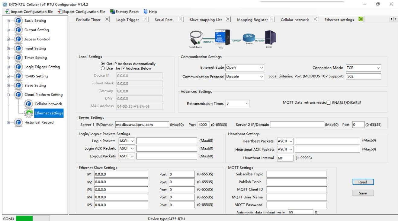
**Get IP address Automatically:** Tick it stands for: the device automatically obtains the IP address in the LAN. Only when the router in the LAN allows the dynamic allocation of IP addresses can be used.
