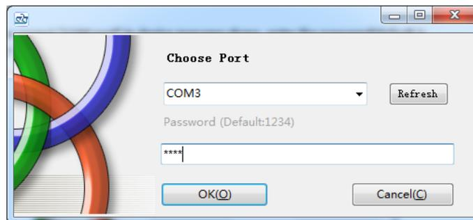
**Tips:** If not connect successfully, will not enter into next step. Pls check if USB connect well, or COM port and password correct or not.
