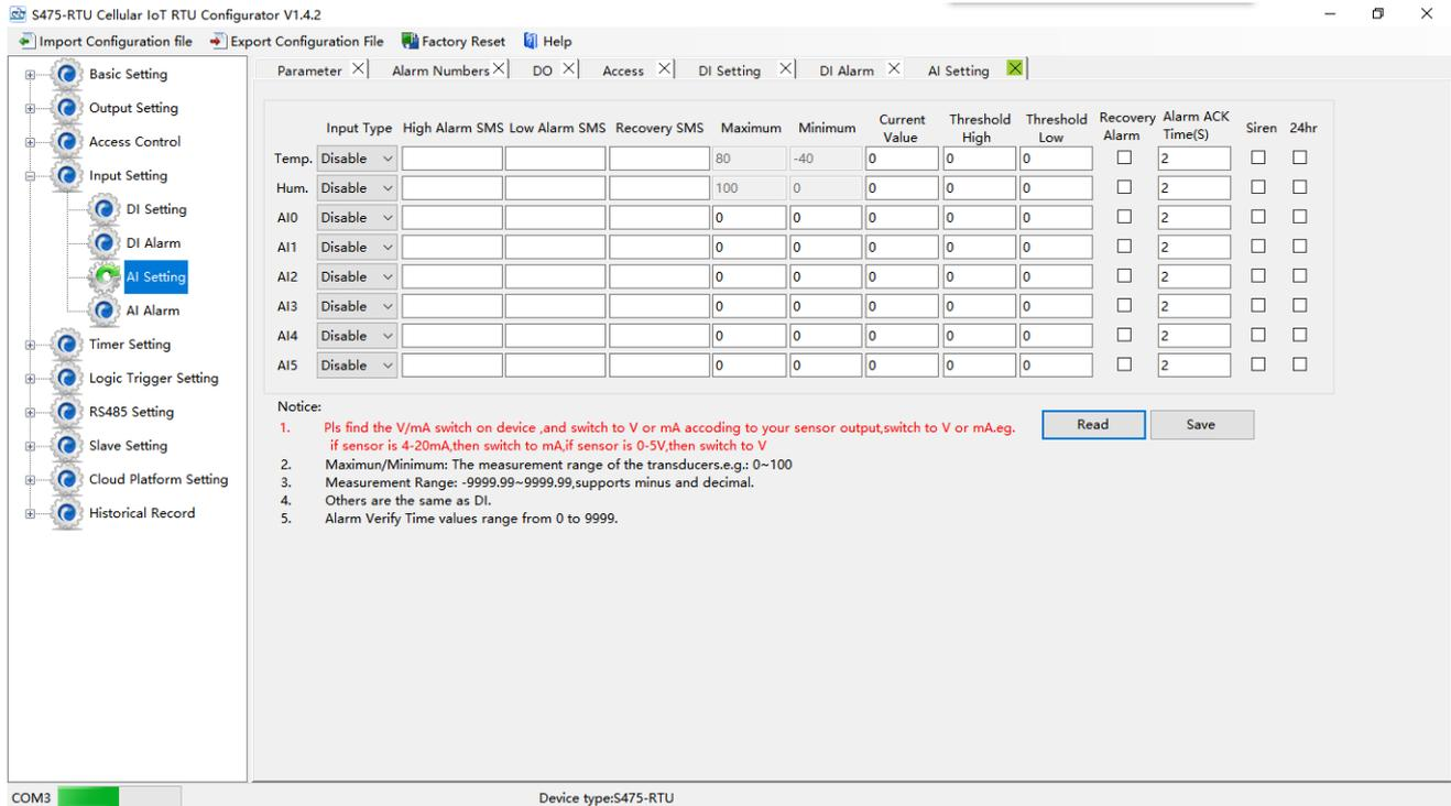
**Input Type:** The user can choose the input type for related channel. Includes: Disable, 0~5V, 0~20mA, 4~20mA.
