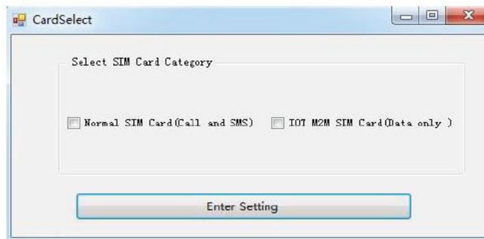
Select the card type of S475 device, the SIM card that supports SMS and phone calls, please select "Normal SIM card", and the SIM card with only data function, please select "IoT M2M SIM card", select "IoT M2M SIM card" and configure The software will disable all functions related to SMS and phone calls.
