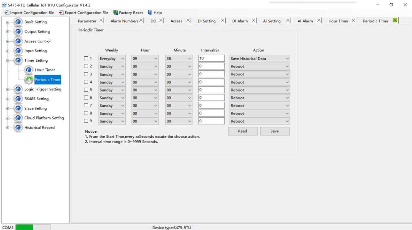
**Weekly+Hour+Minute:** Stands for what day and at what time does the RTU should start to execute the action and interval how many seconds then repeat to execute the action.
